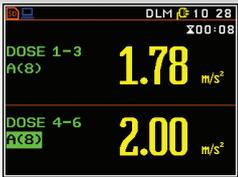
The ISO 5349-2 measurement technique requires simultaneous assessment of frequency weighted RMS values in 3 axes and combining them as a vibration total value. The vibration total value result is a basis for calculation of the A(8) vibration exposure which has a daily limit of 5 m/s<sup>2</sup> in accordance with the Vibration Directive or 400 points in accordance with the UK regulations. Depending on the working activity, the measurement may require assessment of A(8) on one or both hands.
