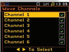
To meet the requirements of ISO 2631-5 the SV106 offers a possibility of recording the raw time domain signal to the WAV format. The mentioned standard describes the dose calculation from the time domain signal in case of multiple shocks.
