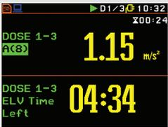
The ISO 2631-1 specifies different weighting filters and indicators for evaluation of effect of vibration on human health, comfort and perception. In accordance with ISO 2631-1 and European Directive the A(8) vibration exposure value is calculated as the highest value of frequency weighted RMS determined in 3 axes including the weighting factor of 1.4 in the X and Y axes.
