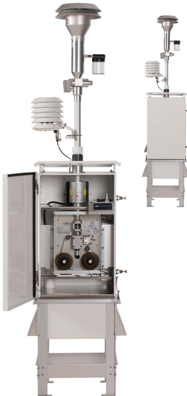
The BAM 1022 has US-EPA designation for  $PM_{2.5}$  (EQPM-1013-209) for which a dedicated hourly output channel is available. A second, real-time output channel will provide the user with continuous PM updates down to 1-minute time resolution. The BAM 1022 is ideal for the following applications:
