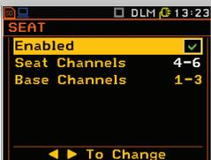
The methods of evaluation of vehicle seat vibration are described in ISO 10326. Following this standard SEAT values are the ratio of the vibration exposure at the seat to that at the floor, where a complete rigid seat would have a value of 1.0. For this application the SV106 is using two sensors the SV38V and SV151.
