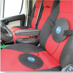
The SV106 fully complies to requirements of ISO 2631-1 and Vibration EU Directive providing the A(8) vibration exposure value referring to health and overall vibration total value (VECTOR) for the evaluation of comfort. Two inputs allow connection of 2 tri-axial whole-body vibration sensors simultaneously.
